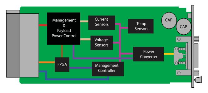
FIGURE 1. UTC011 Functional Block Diagram
